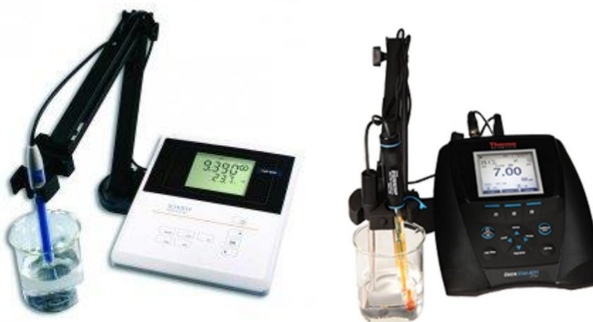
pH-metr Lab 850, SHOTT pH-metr Orion Star™ A211
